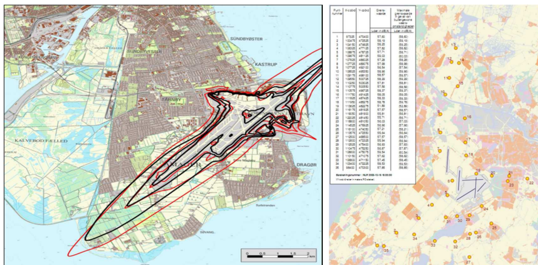
figure 17 Examples of maximum noise contours. Left: Copenhagen airport. The red are the not-to-exceed contours, in black the recently realised ones (year unknown). Right: Amsterdam airport. The yellow circles indicate enforcement positions and the list defines the not-to-exceed Lden levels.
