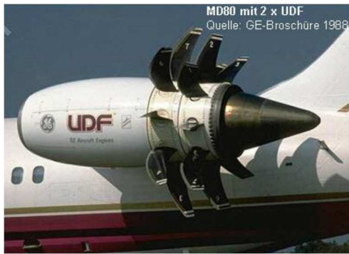
figure 31 Picture of a concept high efficiency engine design with counter rotating propellers.
